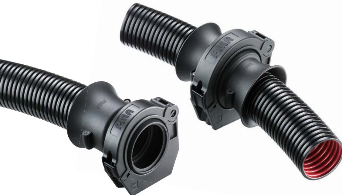
Through different conduit types for various requirements, system supports and a range of special accessories, torsion can be avoided and the stresses upon the cables reduced to a minimum. Special conduit designs, supports and abrasion protection sleeves provide optimal protection along the entire length of all moving elements, enabling engineers to achieve a massive reduction in torsion forces.
