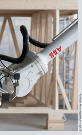
Wooden building modules are pre-fabricated in ETH's Robotic Fabrication Laboratory by two ABB robots equipped with **PMA®**'s cable protection products.
