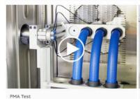
Resistance to Fatigue when Exposed to Continuous Bending 2
