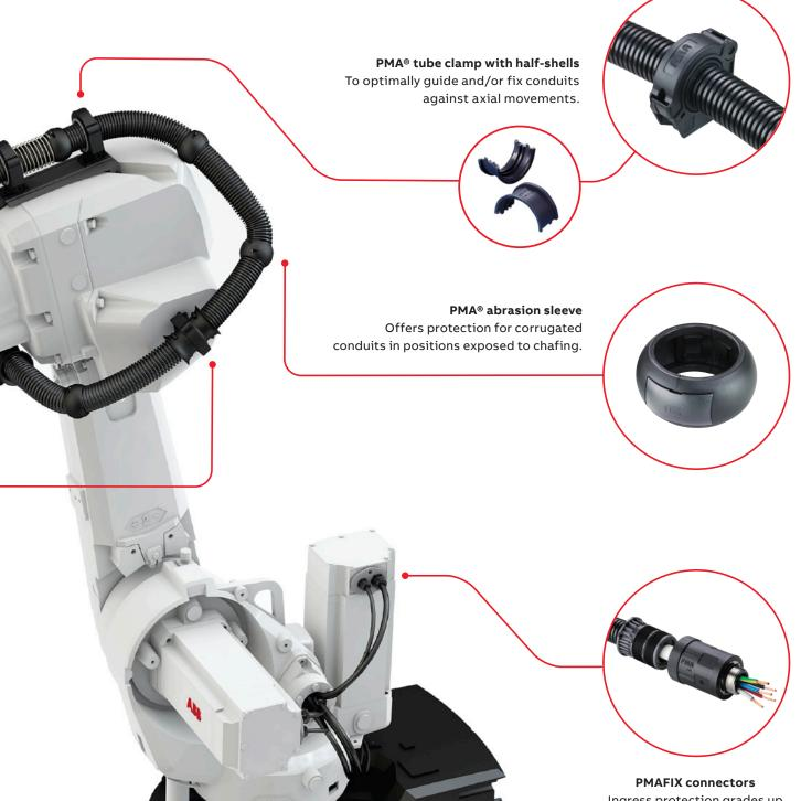
PMAFIX connectors Ingress protection grades up to IP68 and IP69, even in applications where there is long term continuous movement.
